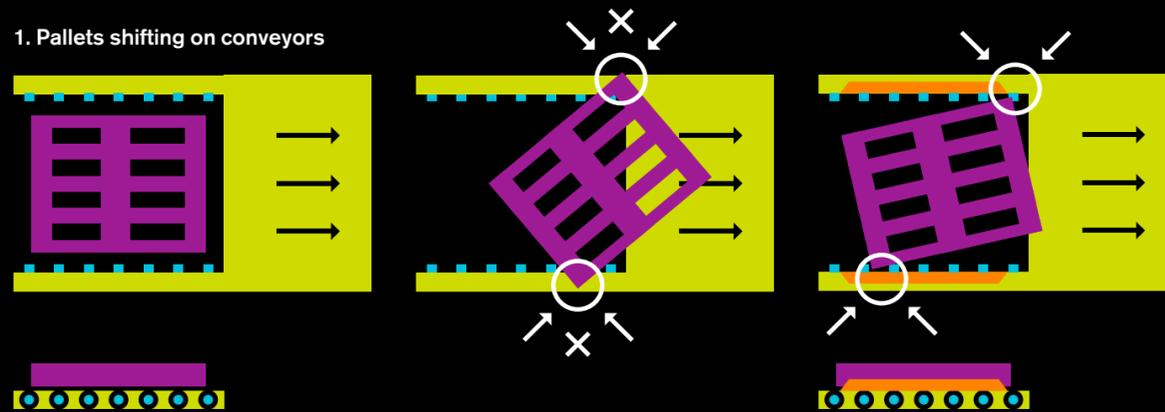
A customer experienced frequent conveyor jams caused by open sides.
